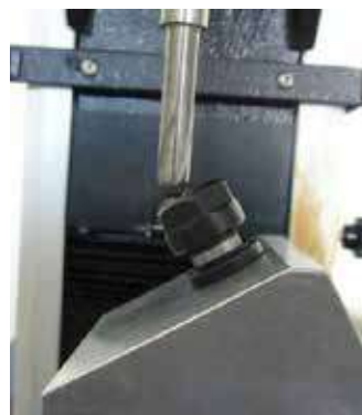
3. Abutment Broken Average Force 1089N
