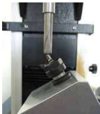
2. Instron Implant-Abutment Fatigue Test ISO 14801
