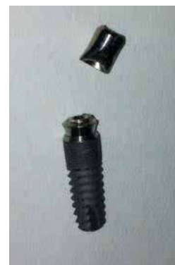
4. Fracture (Abutment Level Broken) Abutment Screw & Implant Undeformed
